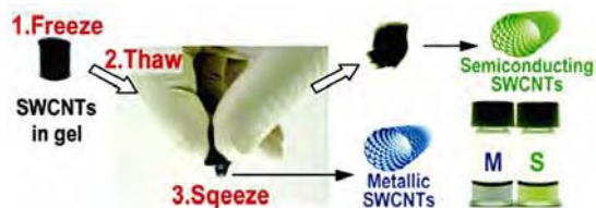
Fig. 14 — Separation of SWNTs by a gel-squeezing method in which a piece of gel containing SWNTs and SDS was frozen, thawed and squeezed. [Reproduced from Ref. 15 with permission from American Chemical Society, Washington DC, USA].
