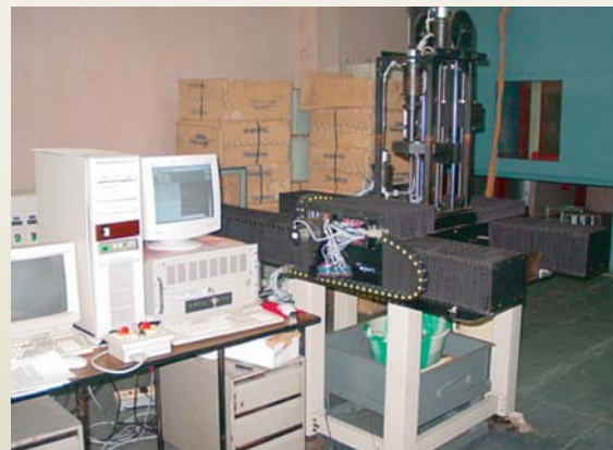
Fig. 3 : C-scan ultrasonic facility at IGCAR
