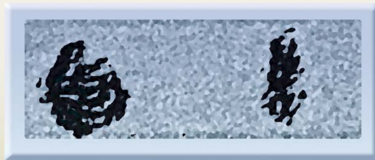
Fig. 5 : C-Scan image of the titanium-aluminum braze plate indicating lack of bond (Black patches).
