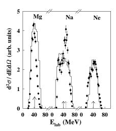
FIG. 2. Exclusive (filled circles) energy spectra for Mg, Na and Ne at  $\theta_{lab} = 15^{\circ}$ . The solid histograms are the statistical model predictions (using code LILITA) and the solid and dashed arrows indicate the energy corresponding to  $v_{cn}\cos(\theta_{lab})$  and the expected fission fragment kinetic energies.
