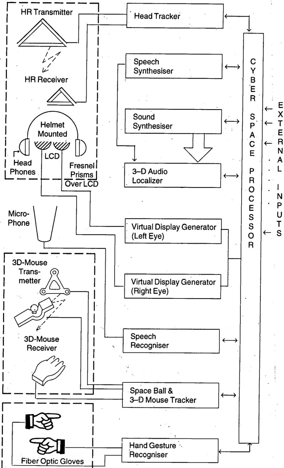
Fig. 1 Components of the Virtual Environment Laboratory of the National Informatics Centre (VELNIC)
