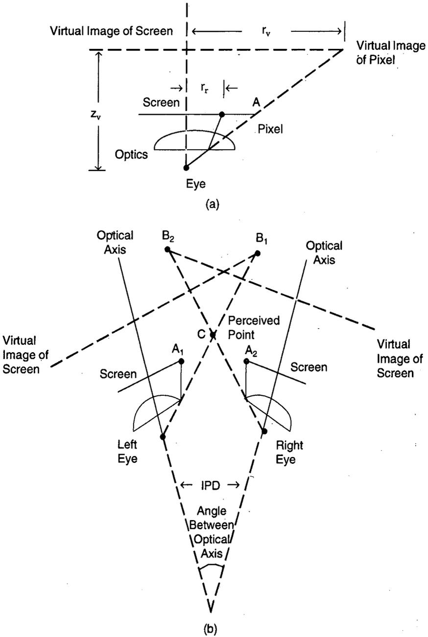
Fig. 3 (a) Single eye optics model and (b) Stereoscopic optics model for the head-mounted LCD display
