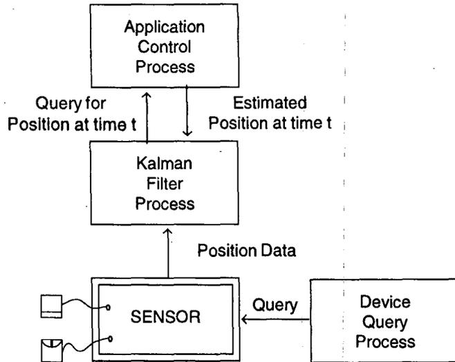
Fig. 4 Communications for control and filtering of a sensor device
