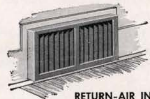
RETURN-AIR INTAKE (for forced system)
