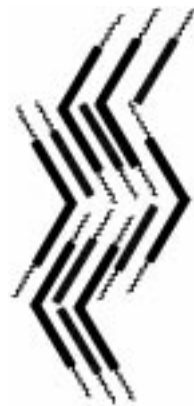
Figure 8. Schematic representation of the structure in the B_6 phase exhibited by mixtures of compounds made of R and BC molecules.
