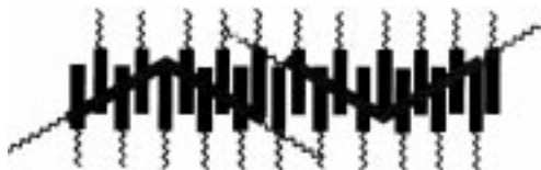
Figure 10. Schematic representation of the structure in the SmA db liquid crystal.
