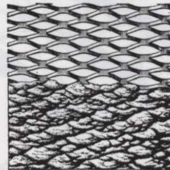
In metal lath, plaster forms small keys.
