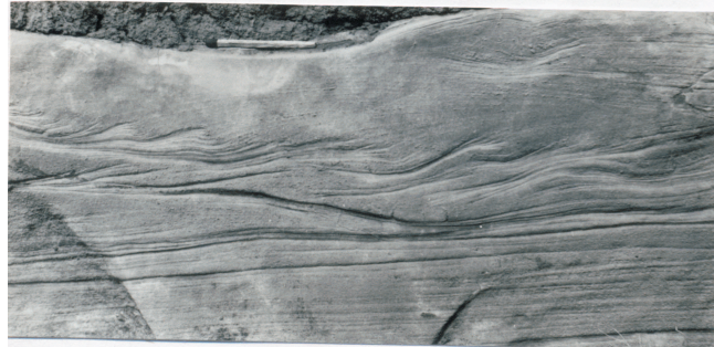
Figure 7. Climbing ripple set gradationally overlying plane laminations in facies D (match-stick length = 4.5 cm).
