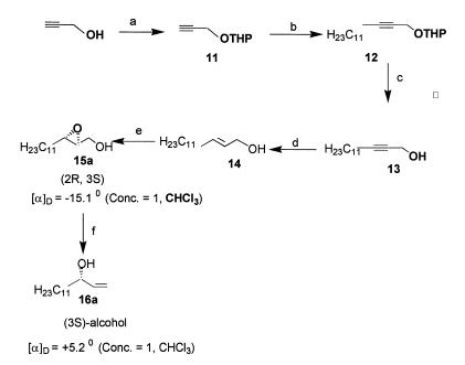
$\begin{array}{l} \textbf{Scheme 3} \text{ Reagents: a) DHP, p-TSA, DCM; b) C_{11}H_{23}Br, Li-Liq. NH_3-THF; c) MeOH-p-TSA; d) LAH, THF, reflux; e) (+)-DIPT, TIP, TBHP, 4A molecular sieves, DCM, -25 °C; f) Cp_2TiCl_2, Zn, ZnCl_2. \end{array}$
