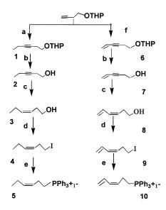
**Scheme 2** Reagents: a)  $C_2H_5Br$ , Li-Liq. NH<sub>3</sub>, THF; b) MeOH, p-TSA; c) Lindlar-H<sub>2</sub>; d) TPP, I<sub>2</sub>, imidazole, benzene, r.t.; e) TPP, benzene, reflux; f) vinyl magnesium bromide, Pd<sup>0</sup> CuI, THF-TEA.
