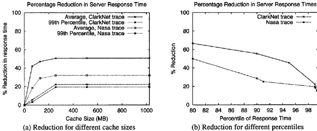
Figure 9: Reduction in Server Response Times due to Caching
