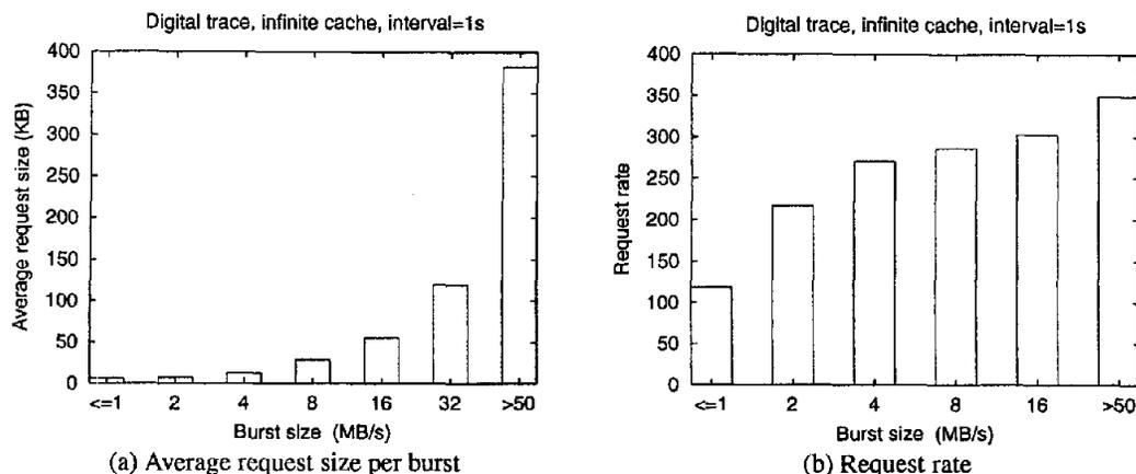
Figure 13: Variation in the average requests size and the request rate with increasing burst size.
