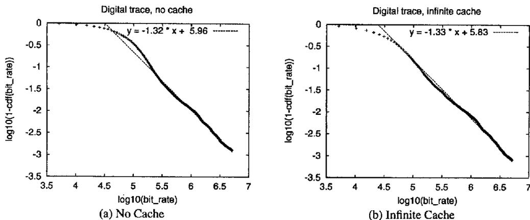
Figure 11: Determination of the  $\alpha$  parameter of the Pareto distribution using LLCD plots.
