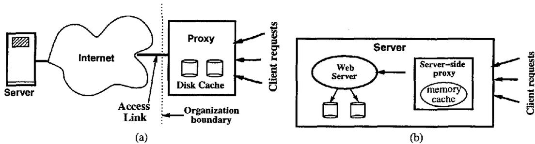
Figure 2: Simulation environments for (a) a proxy near an access link and (b) a server-side proxy.
