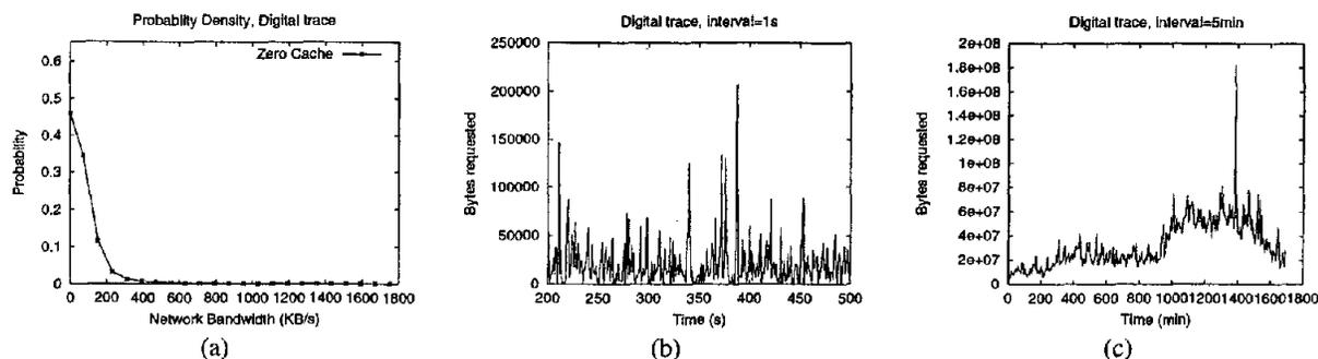
Figure 1: Heavy-tailed and bursty nature of web workloads. Figure (a) shows that the distribution of network bandwidth usage is heavy tailed. Figures (b) and (c) demonstrate the bursty nature of web workloads over time scales of one second and five minutes.
