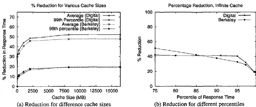
Figure 7: Reduction in response time due to caching
