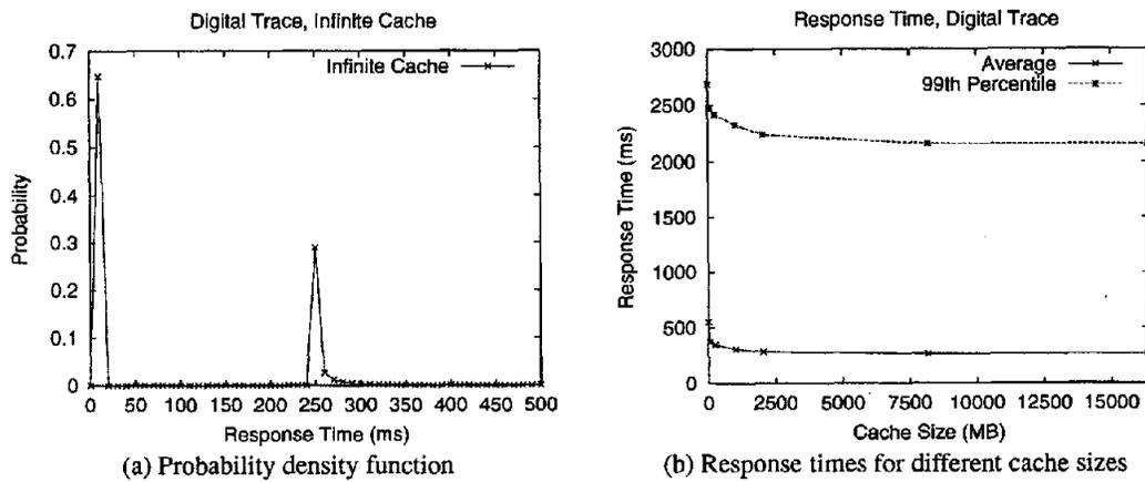
Figure 5: Impact of caching on response times. Figure (a) plots the probability density function of the response time while figure (b) shows the variation in the average and 99<sup>th</sup> percentile of the response time with increasing cache sizes.
