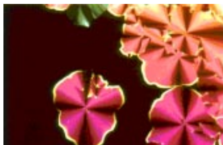
Figure 2. Optical photomicrograph of the hexagonal columnar phase developing from the isotropic liquid, compound 3 , 79.5°C.
