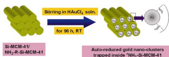
Scheme 1 The probable structure of the NH 2 -MCM-41 material before and after immersion in HAuCl 4 solution for 96 h. The magnified view of the cross-section shows the entrapped gold nanoparticles formed by spontaneous reduction of chloroaurate ions by the MCM-41 material.
