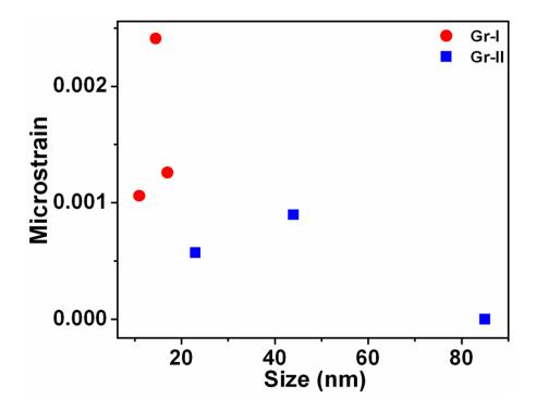
**Figure 3.** Microstrain calculated from XRD data by Williamson-Hall analysis is plotted as function of the size. The relaxation of the strain at the shape transition is apparent.
