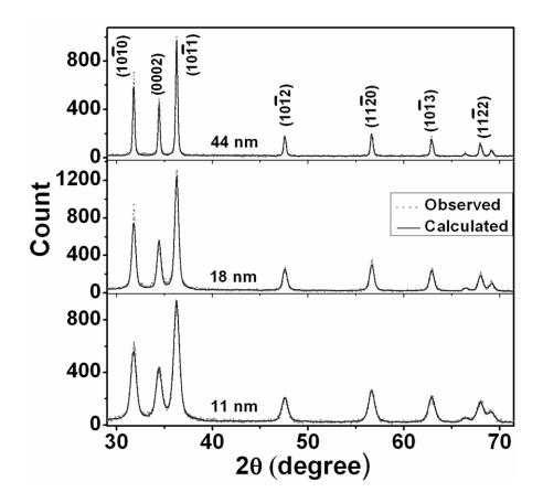
Figure 2. XRD data for select samples as indicated on the graph show wurtzite type structure adopting symmetry P63mc (peaks are indexed).
