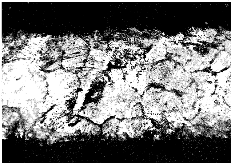
FIG. 9. The cross section of 15/85 In-Ag alloy foil after oxidation in 76 Torr oxygen pressure at 600 °C for 4 h. The unevenness of the surface is due to the external oxide layer.
