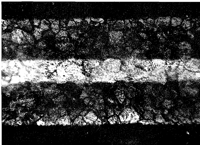
FIG. 7. The cross section of the 5/95 In-Ag alloy foil after oxidation at 600 °C in 76 Torr oxygen pressure for 2 h. The lighter band in the middle is the unoxidized alloy.
