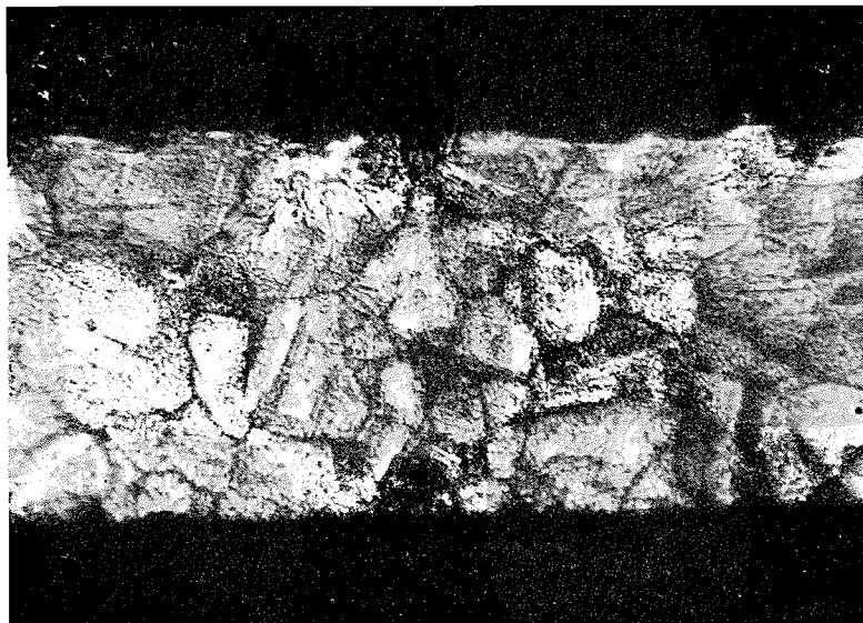
FIG. 8. The cross section of the 10/90 In-Ag alloy after oxidation at 600 °C in 76 Torr oxygen pressure for 4 h.
