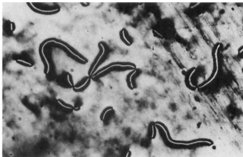
FIGURE 7 An inversion wall of the first kind with a -\frac{3}{2} disclination in a mixture of 12 weight per cent of LQ with p -cyanophenyl- p - n -heptylbenzoate at 28^{\circ}\text{C} ( \times 540 ).
