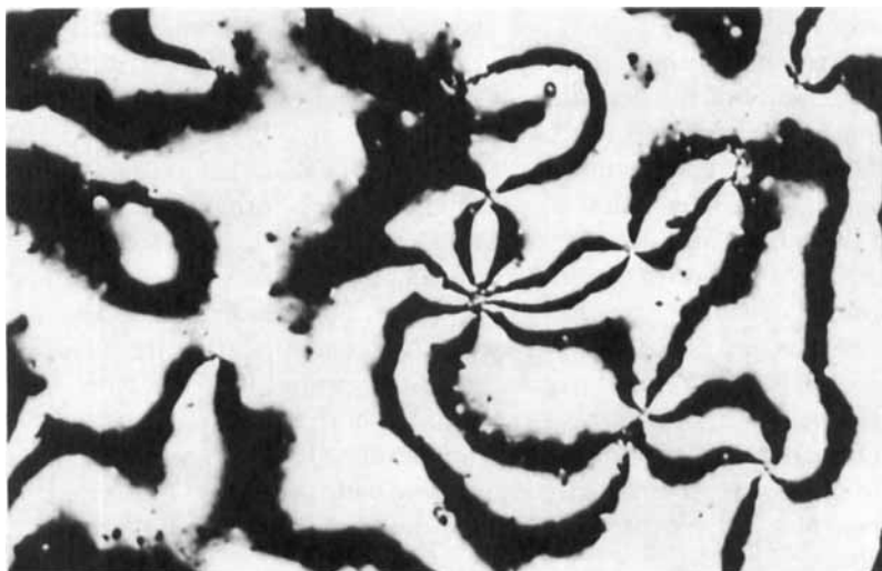
FIGURE 5 A -2 defect in a mixture of 20 weight per cent of LQ with p -octyloxy- p '-cyanobiphenyl at 50°C. Illumination with white light ( \times 540 ).
