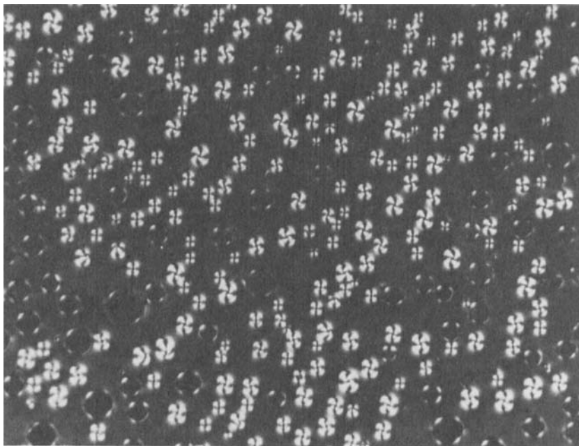
FIGURE 5 A coexistence region between N_R and N_D phases photographed between crossed linear polarizers with \psi = 0^\circ ( \times 570 ).
