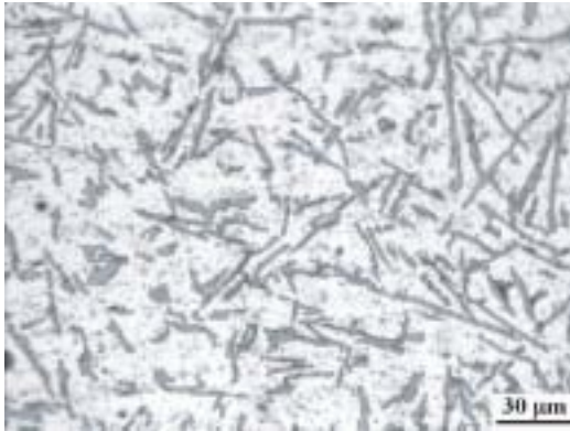
FIGURE 1 Scanning Electron Micrograph of the as-received Al-Si alloy used in the present study.
