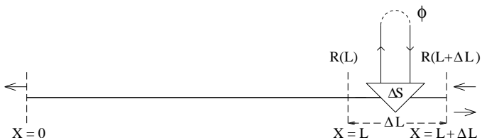
FIG. 2: A schematic description of the ‘invariant imbedding’ method for a 1D conductor with random-phase reservoirs distributed uniformly along the length.
