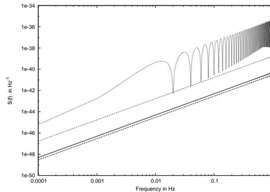
**Figure 3.** The ‘top’ curve shows the PSD  $S_{\alpha}(f)$  of the secondary noises. The straight lines are the PSDs of the residual noise at three epochs chosen an year apart. Clearly the residual laser noise is seen to be adequately below the secondary noises.
