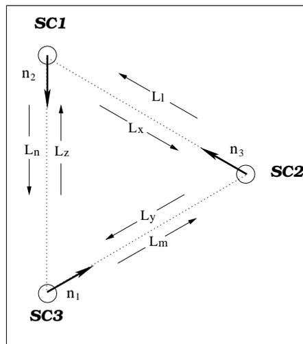
**Figure 2.** A schematic diagram of LISA's optical links.
