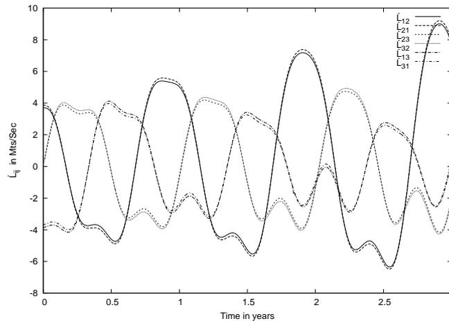
**Figure 1.** The rate of change of armlengths for the six links is shown in units of m/sec for  $\phi_0 = 0$ . This rate of change is less than 6 m/sec up to the second year and increases to a maximum of about 8 m/sec in the third year.
