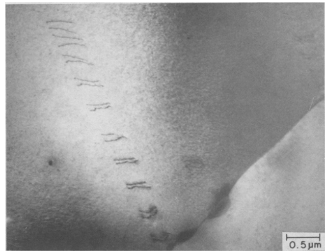
Fig. 6—Planar arrangement of dislocation pairs in specimen aged at 873 K for 2 h.
