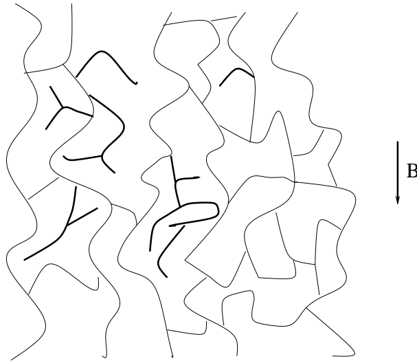
Figure 2. Schematic representation of the percolation cluster with density above the critical threshold. The heavy lines denote the dead-end branches.
