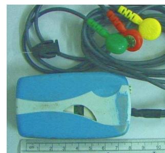
Fig. 1. A picture of the W-ECG developed at IIT Bombay, placed by the side of a 15-cm ruler.
