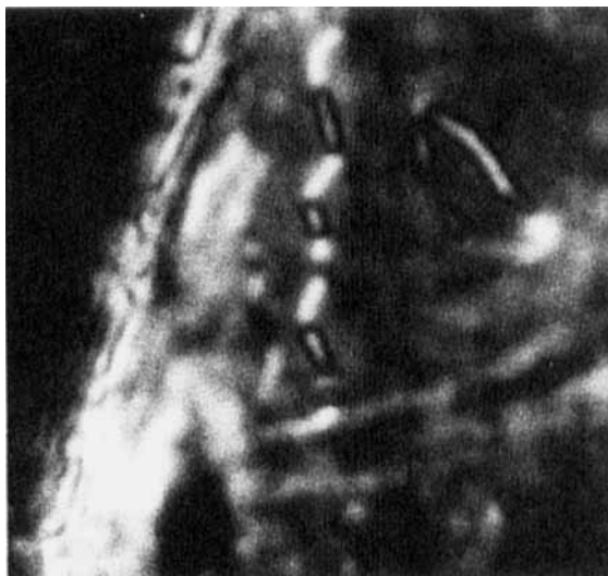
FIGURE 2 Zig-zag disclination in the nematic phase of Complex I with R = \text{OCH}_3 . The disclination, running vertically in the middle of the photograph, consists of alternately bright and dark segments.
