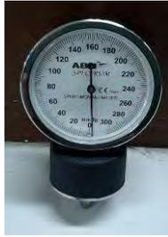
**Gambar C.1** Tensimeter aneroid
