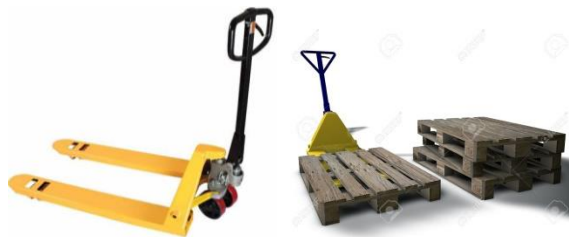
Gambar 5.3 Pallet jack dan loading pallet
