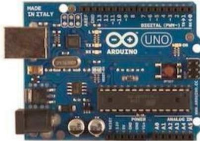
**Gambar 2.9** Arduino Uno (Margolis, 2011)
