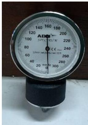
**Gambar B.4** Tensimeter Aneroid
