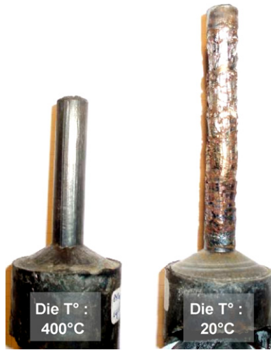
Fig. 9. Thixoextruded parts forged using a “cold” die and a “warm” die (ram speed 215 mm/s, initial slug temperature 1445 °C).
