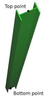
Figure 8: The top center point and bottom center point of a column typically used as control point for dimensional control.
