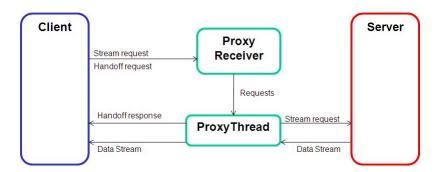
Figure 4.3: Flow of requests from the client, proxy and server
