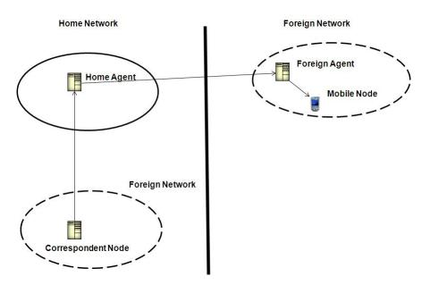
Figure 2.6: Components of MobileIP
