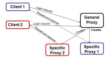
Figure 4.2: Proxy and client interaction
