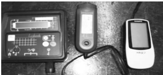
Figure 1: The sensing kit; Science Scope data logger with an external sensor attached, and a Garmin GPS
