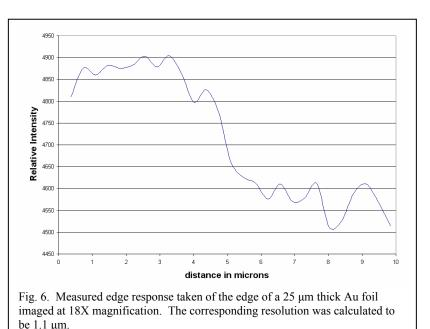
detector pixel size can be calculated at M = 18.4 as 6.7  $\mu$ m x 2 / 18.4 = 0.73  $\mu$ m. Here we assume at least 2 pixels are needed to resolve an object. The use of parabolic lenses and some form of filtering of the source are essential to improving image resolution. Earlier we reported 6-um resolution with a spherical bubble
