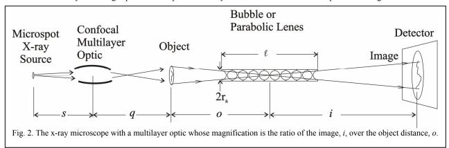
maximum possible x-ray flux to a 200  $\mu$ m spot with minimum divergence. The optic has an approximately 1 mm x 1 mm output aperture and focuses to a spot 38 cm away from the optic. Importantly, the local divergence at each point of the output is approximately 1 mrad, which is sufficiently to fill the aperture of the CRL for each point on the object. If the divergence were too small, not enough x-rays would be collected by the lens to form an image.
