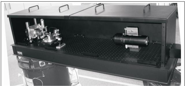
Fig. 7. Picture of the portable tomographic imaging system. The source, x-ray optic, rotation stage and CRL are located on the left; the x-ray camera is on the right. The drift space from the CRL to the camera is to achieve a magnification from 4 - 10 X depending on the configuration. The side panel shielding was removed for the picture. The system also includes a separate rack with the control system and power supplies.
