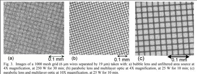
source and CRL, 6-µm wires are clearly resolved and with much greater contrast. Indeed, even at 2.5 times greater magnification the contrast improved over the previous system.
