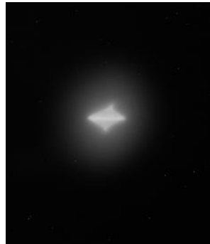
Fig. 4. Demagnified ( M = 0.2 ) X-ray tube focal spot image taken with lens #2 and the X-ray micron resolution CCD camera.
