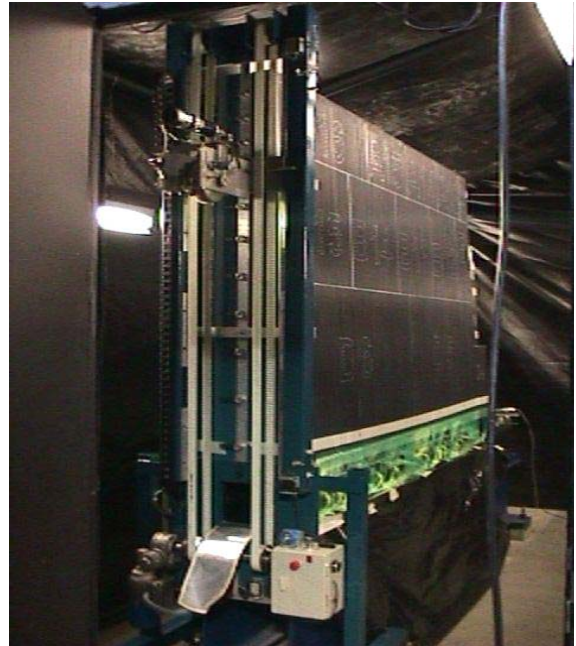
Fig. 14. Two instrumentation areas at the IFAE-Barcelona workshop. On the left, module IFA08 is being instrumented. On the right, module IFA07 is placed in a dark room and is being certified with the movable LED light source system.
