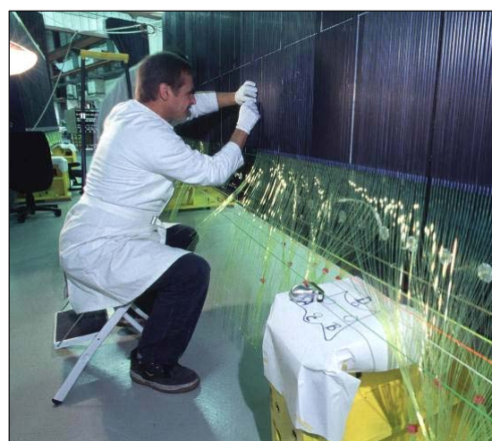
Fig. 8. Inserting tiles and profiles with fibers into a Barrel module
