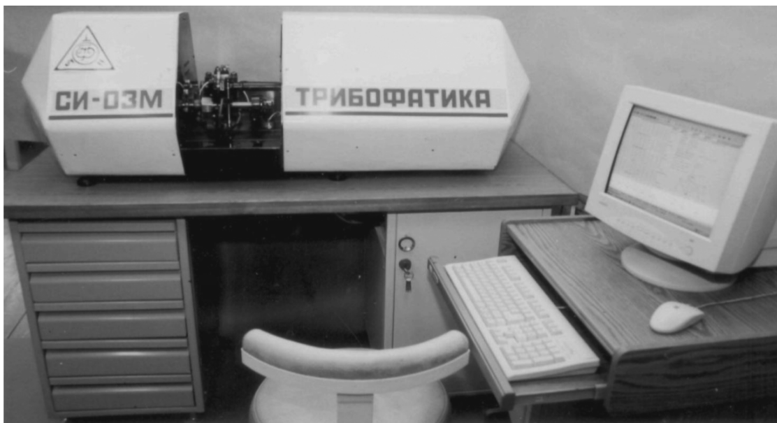
Fig. 3. General view of SI-03M universal test machine for wear-fatigue tests.
