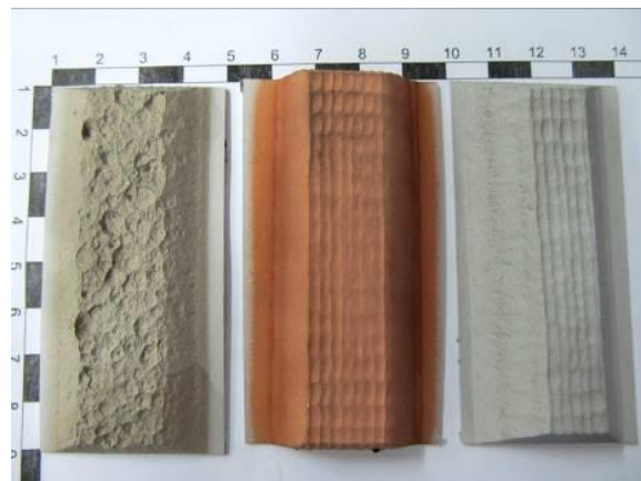
Fig. 3. As deposited bulk samples (NiFe, CuFe FeAl, from left to right). (full colour version available online)
