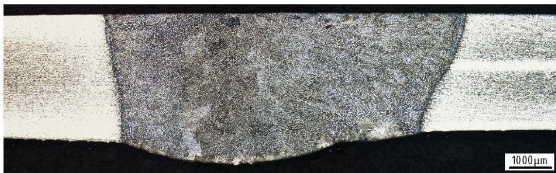
Fig. 6. Corrosion attack of the specimen with ground surface.
