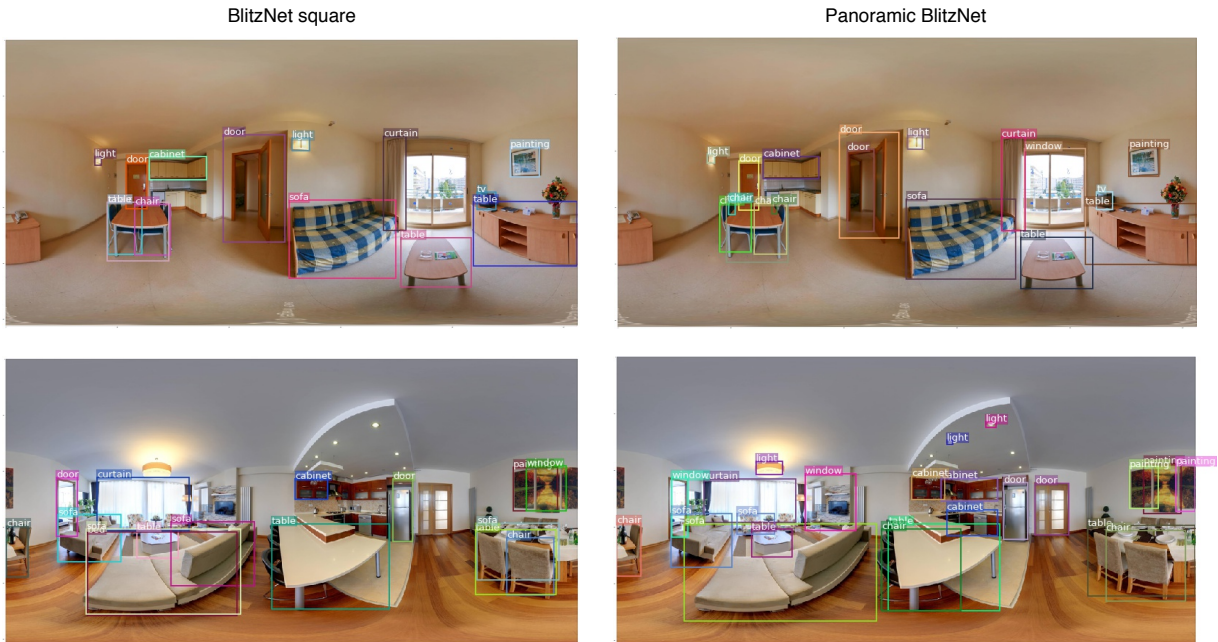
Figure 5.2: Qualitative evaluation of object detection: BlitzNet initial model (squared images), and Panoramic BlitzNet are compared in these two example images. Second image is complex as having many different objects and bigger distortions. Notice how detection task works well in both models but initial BlitzNet does forget some of the objects and is also less precise in localization of bounding boxes.
