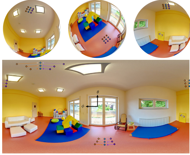
Figure 2.16: EquiConvs kernel on 360° images. Notice the three different kernel positions both projected on the sphere and on the equirectangular image, that highlight differences between offsets depending on the case [14].
