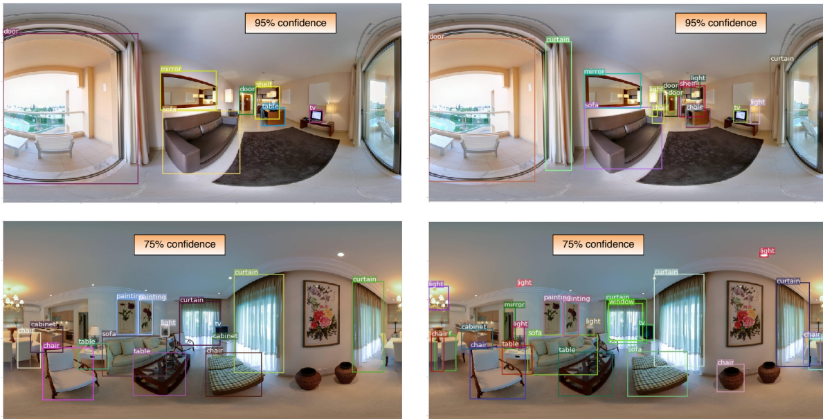
Figure 5.5: Qualitative results of object detection with both standard (left) and equirectangular (right) convolutions, with high confidence thresholds. Notice how EquiConvs detect many more objects (most of them correct) than StandardConvs given the same confidence threshold. Also EquiConvs are slightly more precise on localization bounding box, as seen on the main chair and table of bottom image.
