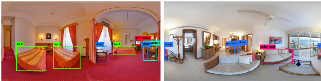
Figure 5.1: Qualitative YOLO experiment results. See very good qualitative results on left image and worse performance on right image, where more distorted objects (sofa, table...) are not detected. Notice how detections are correct in general (high precision) but many objects are not recognized (low recall).
