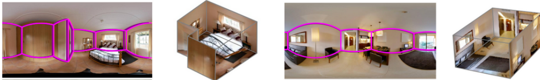
Figure 2.15: Examples of 3D layout recovery task. As seen on the image, they extract edges and corners on the 2D image to conduct 3D reconstruction of the room layout. Figure is taken from results of [14].
