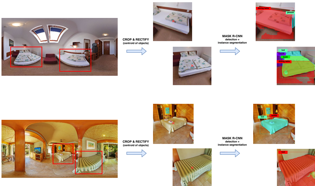
Figure 3.5: Examples of failed segmentations with Mask R-CNN. Images were first cropped and rectified centered on the centroid of each object and given as input for Mask R-CNN Network. Notice wrong segmentation results.
