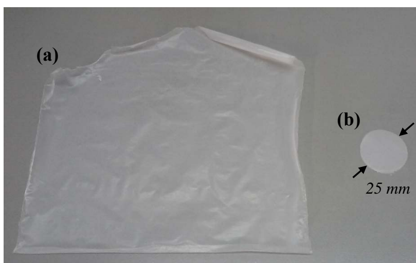
Figure 8. Membrane samples: (a) Membrane after the casting process and (b) Membrane with the optimized size for the permeation measurements
