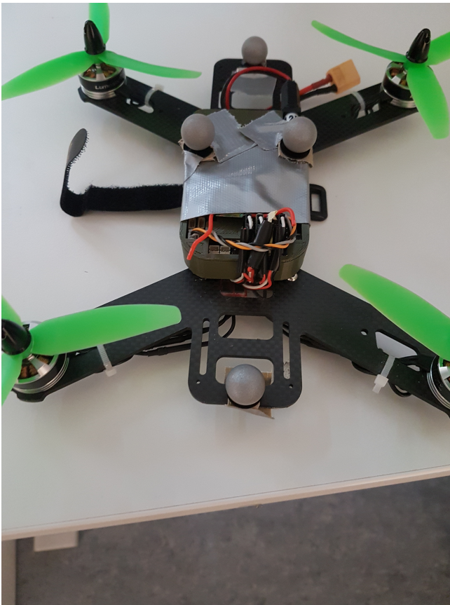
Figure 4.7 The quadcopter equipped with highly reflective silvery spheres, used by the camera system to detect objects.
