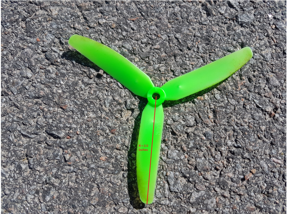
Figure 2.2 Propeller with a 2.5 inch radius \rightarrow 5 inch diameter
