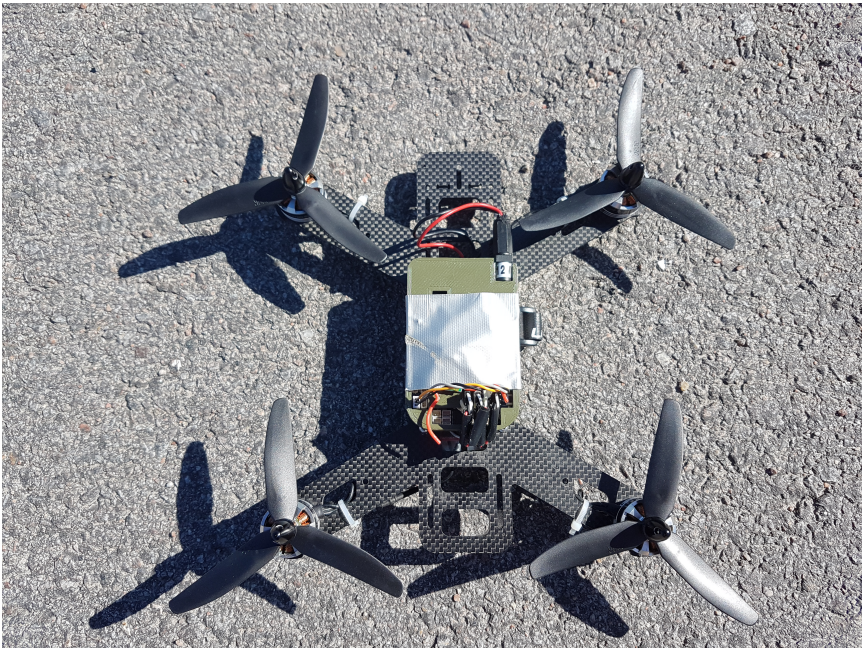
Figure 2.1 The quadcopter platform used in the thesis. The microcomputer can be found inside the green protective case. As the case was not equipped with any form of locking mechanism a bit of duct tape came in handy.
