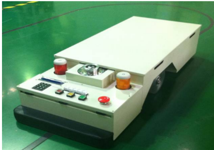
Figure 3.12 - An AGV following a magnetic strip (Ecvv.com, 2017)
