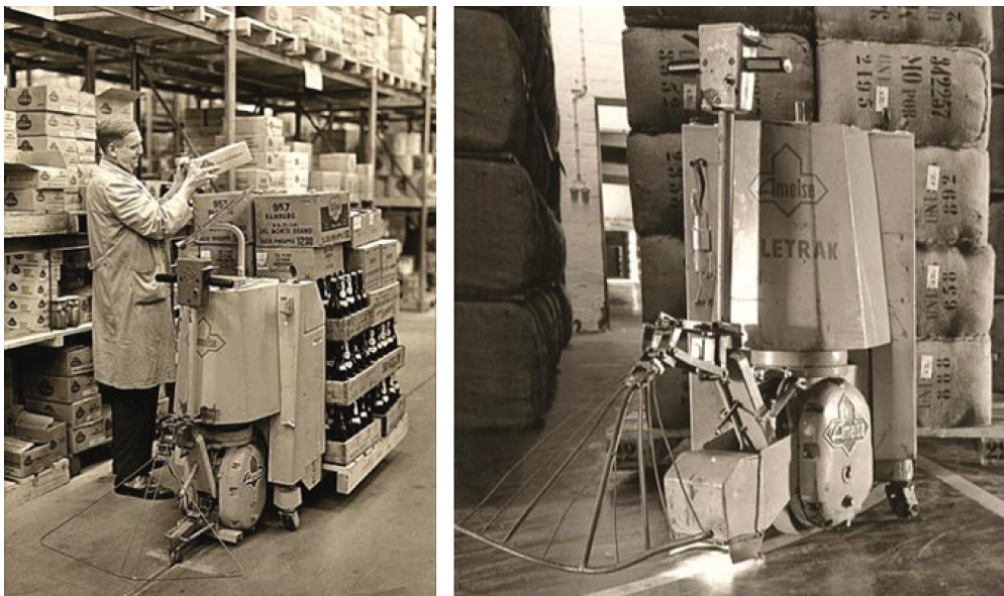
Figure 3.17 - AGVs with wire mesh as bumpers from Ameise and Teletrak (Source E&K (1965) according to Ullrich (2015, p.3)
