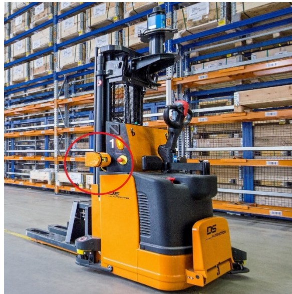
Figure 4.5 - SKF's AGV with two additional sensors at the side (Schmid, 2017)
