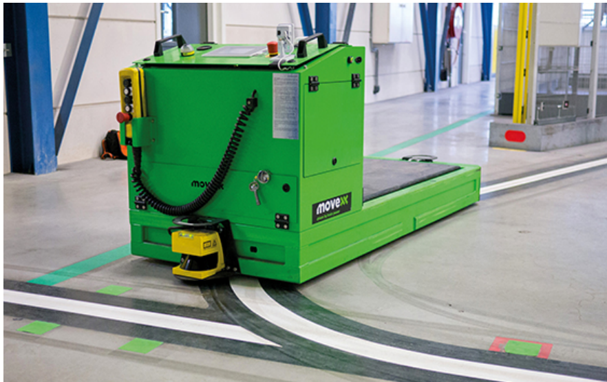
Figure 3.10 - The AGV uses optical guiding to follow its path, and RFID tags to handle more complex situations (Turck.de, 2017)
