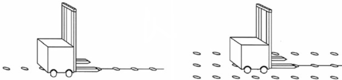
Figure 3.14 - To the left a magnet spot navigation in series, to the right magnet spot navigation in a grid (Ullrich, 2015 p.112)
