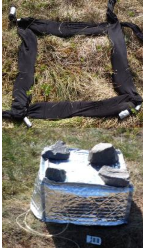
Figure 6: The top picture shows how the pantyhose was put on the ground to fill out any unevenness. The picture below is how the setup looked like, with stones on top to make sure the covering of the chamber was on to suppress the photosynthesis during high speed winds.
