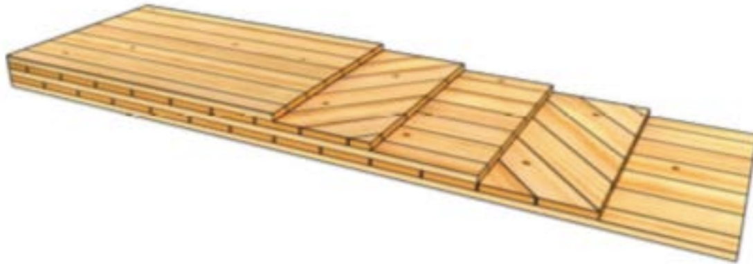
Figure 4-2. CLT with alternating 45° layers
