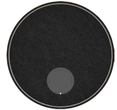
Fig. 219 The Project settles on having the diode recessed into the edge of the orifice.
