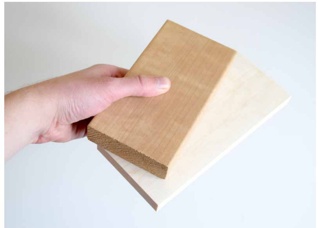
Fig. 206 Visual comparison between Thermally Modified Aspen and Non-treated Aspen.
