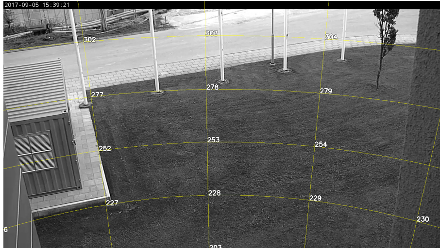
Figure 2.6: Cell generation for PTZ camera from our implementation shown inside camera stream. Mechanical limitation is -180^\circ \leq \text{pan} \leq 180^\circ and -90^\circ \leq \text{tilt} \leq 0^\circ . 25 cells was generated in pan direction and 13 in tilt direction yielding a total of 325 cells. Only a subset of all cells is visible.
