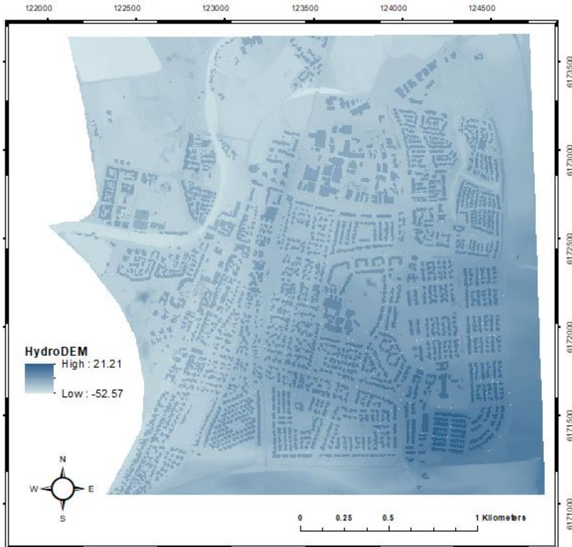
Figure 19 HydroDEM with sink cells unfilled and elevation of buildings raised during DEM pre-processing step. Walls were created around the building polygons and the area bound by the walls was filled in Arc Hydro Tools. This output was converted to ASCII format in order to use it as input DEM to run TFM algorithm in Matlab.
