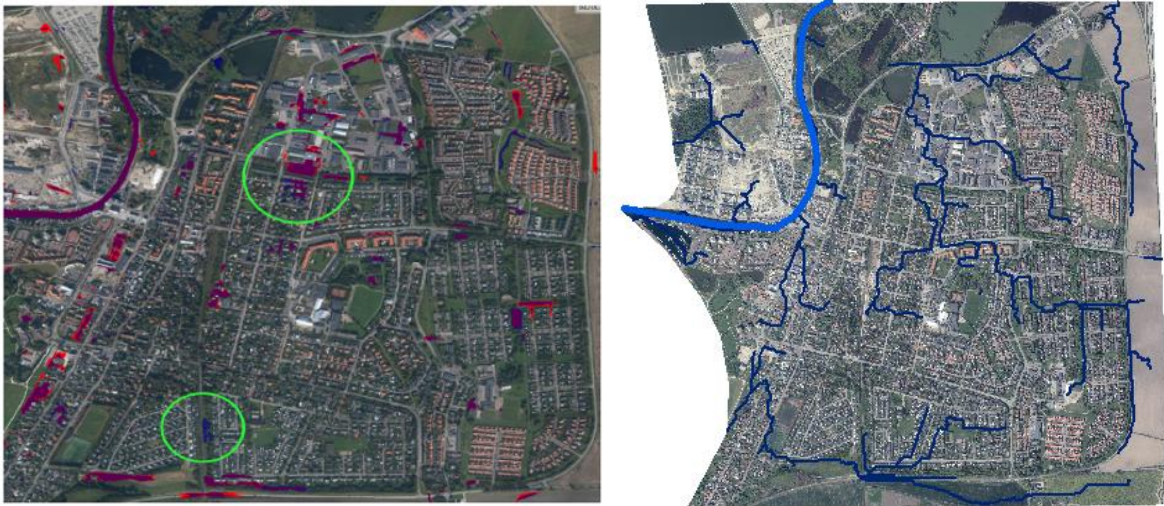
Figure 37 Visual comparison of flood inundated areas by D8 method in this study (right) and HEC-RAS model (left) after 2 hours of simulation (Source: Betsholtz and Nordlöf, 2017).
