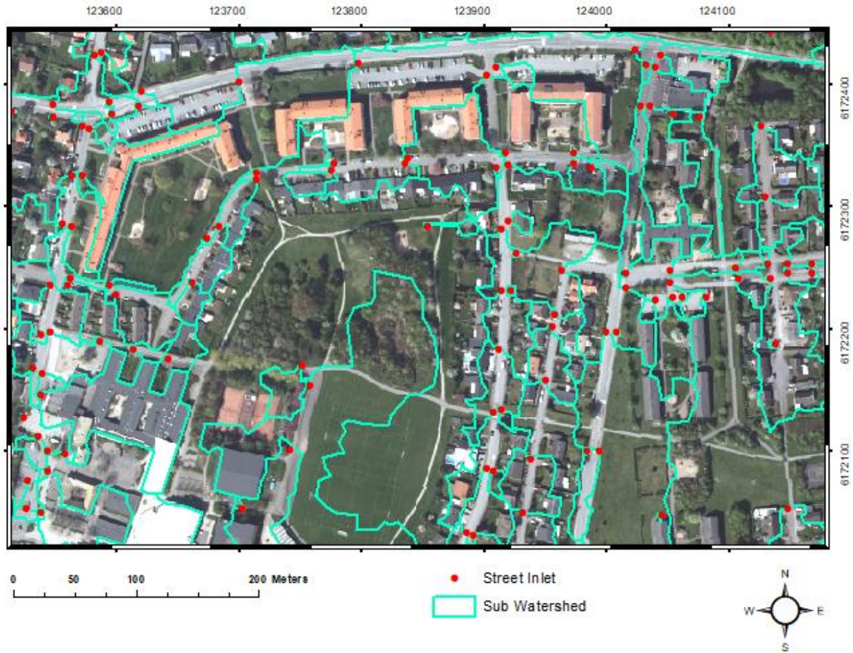
Figure 22 Detail of the study area showing sub-watershed polygons (blue lines) overlaid with Ortho photo, with street inlets as pour points marked in (Red points).
