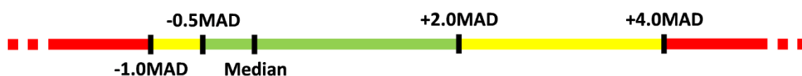
Figure 4. Threshold analysis; limits for the three thresholds; GREEN, YELLOW and RED, as intervals about the median created by \pm numbers of MAD (median absolute deviation).
