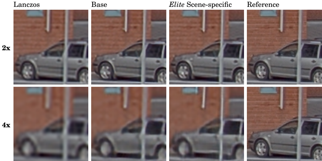
Figure 18: 2x and 4x reconstruction of an unfamiliar scene, 100 \times 100 pixel samples. From the left: Lanczos filter, Vger base model, Vger Elite scene-specific model, reference image.
