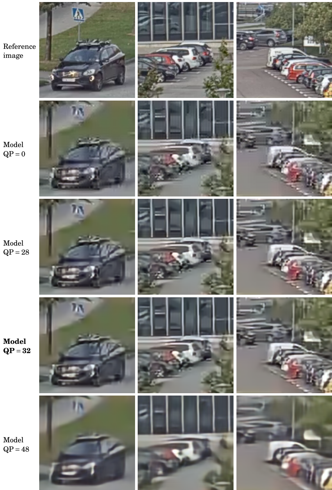
Figure 20: Sample 2x reconstructions of heavily compressed images using the same method as in Figure 19. The reference image has been downscaled by a factor 2 using Lanczos filtering, then H.264-encoded at QP = 40. The figure shows 2x reconstructions with various scene-trained models. Note that model QP = 32 is suggested by Figure 19 to be optimal for video QP = 40.
