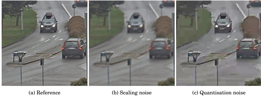
Figure 3: The reference image (a) has been separately degraded by (b) downscaling to half size and then back up again with bicubic filtering, and (c) H.264 encoding at QP = 45. The signal loss in (b) and (c) is about equal when measured in peak signal-to-noise (see section 3.6.1).
