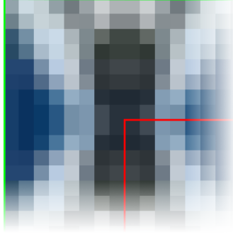
Figure 5: 8-pixel even reflection of an image, top-left corner. The red and green lines mark the image boundary before and after reflection, respectively.
