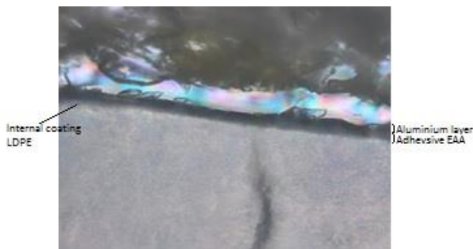
Figure 16: Cross section of a peeled strip from the pre-experiment simulant 1 showing the Al surface after 44 days. The scale bar has been lost, but as an indication of size, the aluminium foil is known to be 6-9 \mu\text{m} thick.
