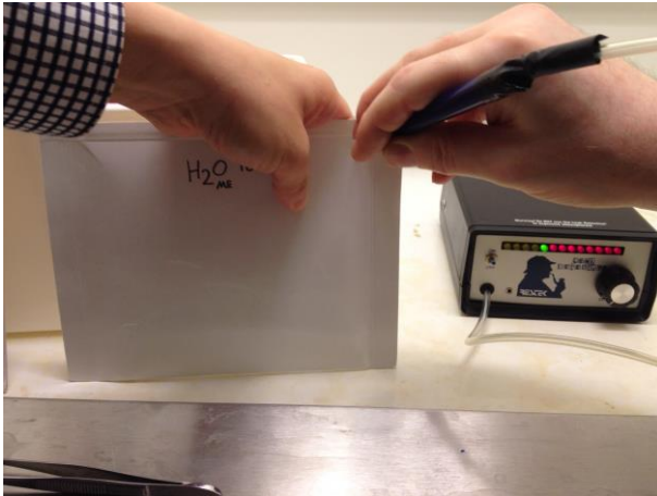
Figure 19: The Leakdetective from Restek Corporation showing a full scale detection of H 2 or He when measuring on the simulant 1 sample from day 36 of the main experiment.
