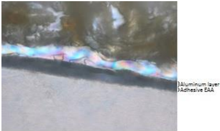
Figure 24: Cross section of a peeled strip from the Main experiment simulant 1 showing the Al surface after 28 days. The scale bar has been lost, but as an indication of size, the aluminium foil is known to be 6-9 \mu\text{m} thick.
