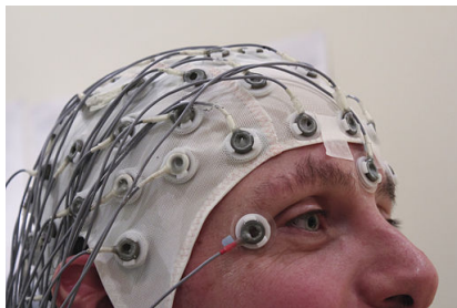
Figure 1.1 A cap used for EEG measurements. The measurements are read from a series of electrodes placed evenly over the head. Taken from http://www.flickr.com/photos/tim_uk/8135755109/ .
