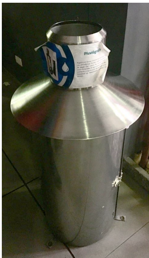
Figure 1: A pluviometric measurement station that IDEAM uses in order to gather information about rainfall.
